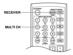
The multichannel input is for connecting a component with individual 5.1-channel analog audio output jacks, such as a DVD player or MPEG decoder. See page 27 for hookup information.
